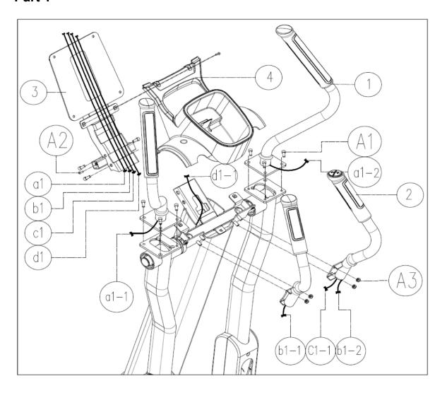
Step 1: as shown in the above figure, first attach (left and right moving handles) with A1 (M8\*16 cylindrical head socket head cap screws) on the mainframe, and pry out the a1-1 and a1-2 terminals;
