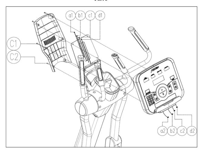
Fix the front and rear plastic parts on the main frame with C1 (M5\*10 semi-circular head cross-stitch screws) and C2 (ST4.2\*12 cross-flowered semi-circular head self-tapping screws).
