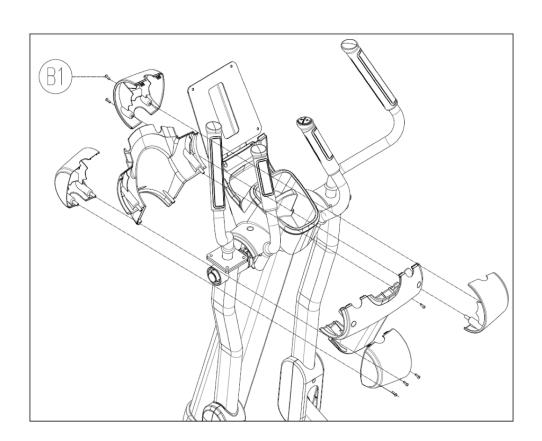
As shown in the figure above, use B1 ST4.2\*12 cross-flowered semi-circular head self-tapping) to fix the plastic parts at the armrest of the boom to the main frame.
