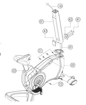
cross self-tapping ST4.2\*12) and C2 (cylindrical head hexagonal screw M6\*12).
