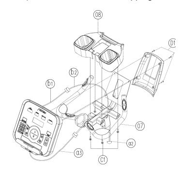
Step 1: Connect the a1 cable in the main frame with the a2 cable on the console. Use A1 (cylindrical head hexagonal screw M10\*85), A2, A3 to connect the assembled head post to the frame tube.
