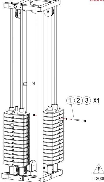
If 200Lb weight stack,use M10X135 bolt in place of M10X170 bolt
